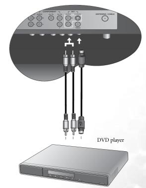
An S-video signal provides a higher quality image to that of Composite video. It is recommended to use this input whenever possible. If your AV equipment provides a component video output (YPBPR or YCBCR), this should be used in preference to either composite or S-video signals.
